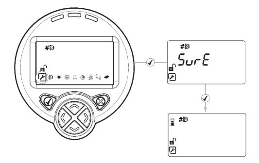
If it is not known where the beam is pointing, use Home Position to automatically steer the infrared beam to approximately the centre of its range of movement.
