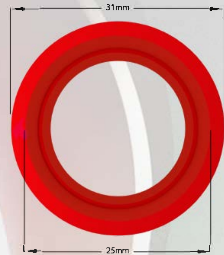
Jointing Socket Front Elevation
