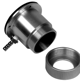
Duct Mount Assembly Stainless Steel – P/N 226846-008 Aluminum – P/N 226846-001 Designed for mounting combustible sensors to air handling duct work (flat surface mounting only).
