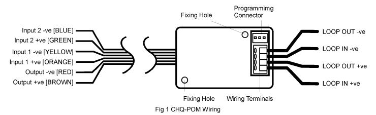
The unit can be fixed to most fixing surfaces with two screws (not supplied) by utilising the two fixing holes (see Fig 1).
