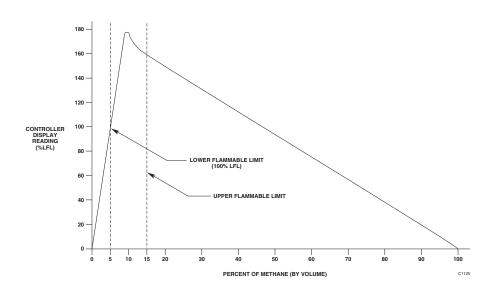
Figure 2—Typical Response of a Catalytic Sensor over a Range of 0 to 100% Methane by Volume
