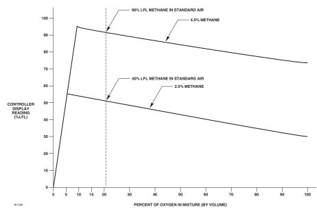
Figure 3—Effect of Oxygen Enriched and Deficient Atmospheres
