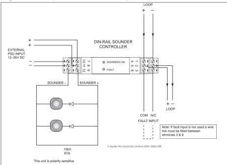
Fig 1 - Wiring diagram for the Sounder Controller
