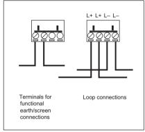
Fig 2 Terminal block connections
