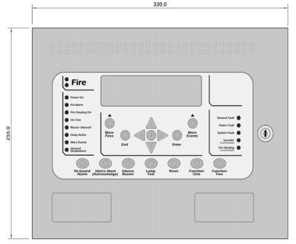
View repeaters have a low standby current consumption and can be powered by the Aux 24V output of the Syncro ASM control panel. For full details of Syncro View repeater units refer to manual MAN-1092.
