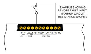
The line impedance should be less than 50 ohms for reliable operation.
