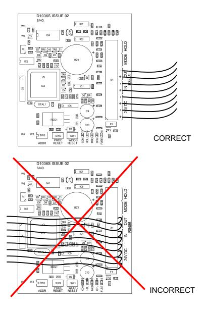
Figure 5. Wiring to the circuit board
