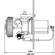
Figure 1—Dimensions of Duct Mount in Inches (Centimeters)
