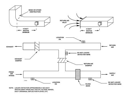
Figure 4—Detector Location Options within the Duct
