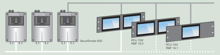
Up to 100 SecuriSmoke ASDs can be shown on a RCU 700. The assignment can be freely selected according customer wishes and the project.
