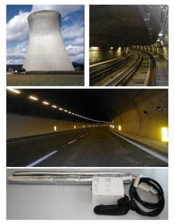
It's possible to use the Thermofibrotester without disassembling the installing clips\* and it works with all kind of fiber-optic cables and Distributed Temperature Sensing systems\*\*. ThermofibroTester is equipped with a carrying case.
