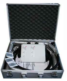
devices are in-built to improve the personal safety during use. Electrical connections are carried out by flexible cables protected against mechanical damages by resistant outer jacket. The flexible cables have specific connectors to plug in easily to the control circuit.
