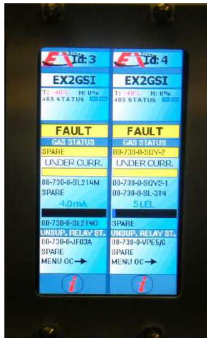
Fig. 12: EX2GSI fault for open line condition on a input channel
