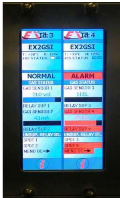
Fig. 11: EX2GSI in alarm condition
