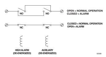
Figure 1—High Alarm and Auxiliary Relays Configured as a De-Energized Pair
