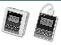
The two rows of large push buttons enable the user to log ON and navigate through the menu trees to the various command and parameter setting functions. The top row of keys are called "Soft Keys" and are assigned programming options appropriate to the screen being viewed.
