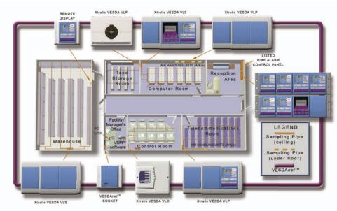
Having all VESDA smoke detectors on a VESDAnet loop allows you to configure and interrogate each detector from a central location, in this case the Facility Manager's office.
