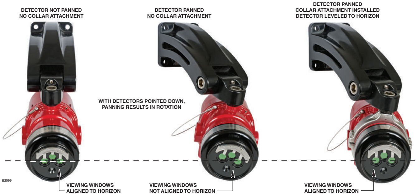
Figure 1—X3301 Detectors Mounted with and without Collar Attachment
