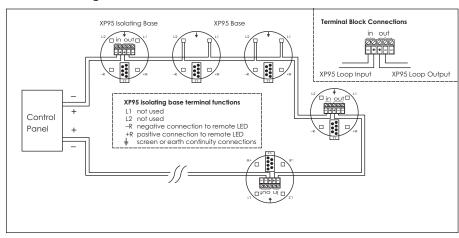
For a full technical specification of XP95 Isolators and isolating bases, please refer to the XP95 Isolators and Isolating Bases PIN Sheet, PP2090.
