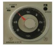
The timer is reset when the switch is turned off and will run for the set period when the switch is turned on again.
